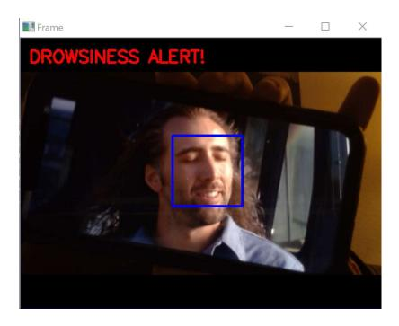
If the drowsiness detector detects a face and the eyes of the user have been closed for more than a few seconds, the user is alerted with a message they are drowsy and an alarm will sound for a few seconds.
