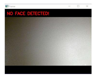
If the drowsiness detector does not recognize a face in the webcam, then it will alert the user that no face is detected.
