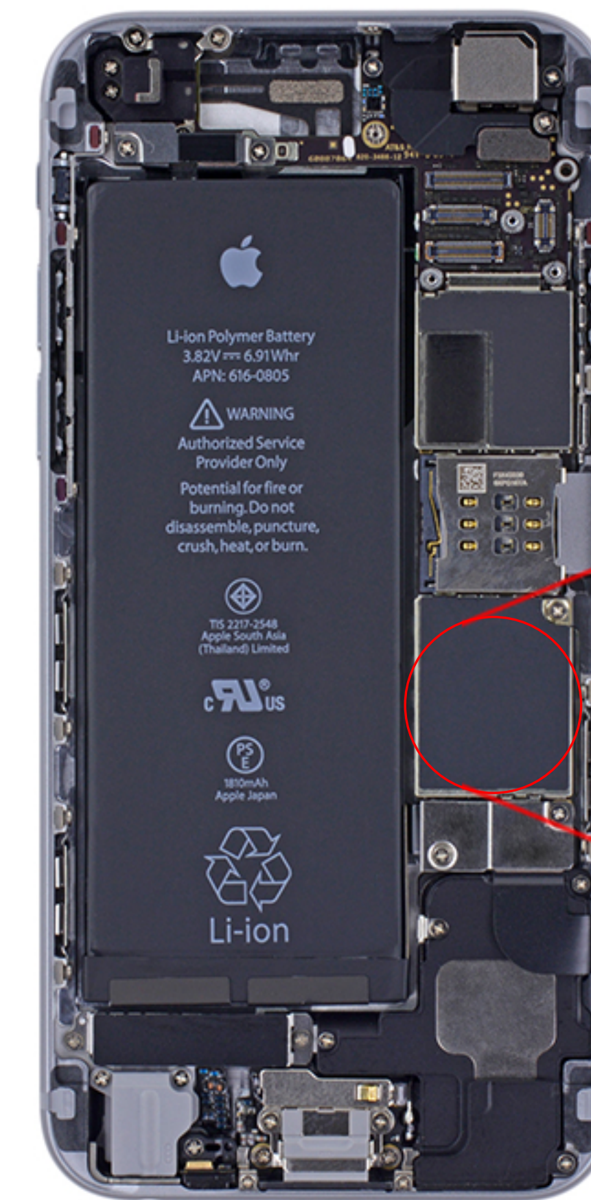
iPhone 6's Bosch BMA280 accelerometer (above), and invenSense MPU-6700 gyroscope (below).
