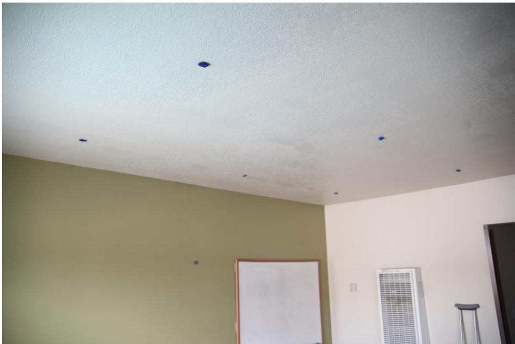
Figure 12: Our bluetooth beacon setup so far in an apartment. There are 7 beacons total: 6 on the ceiling and one on the wall.
