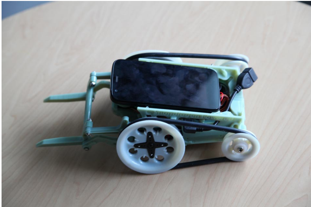
Figure 11: The rover carries the phone, connected through a USB cable.
