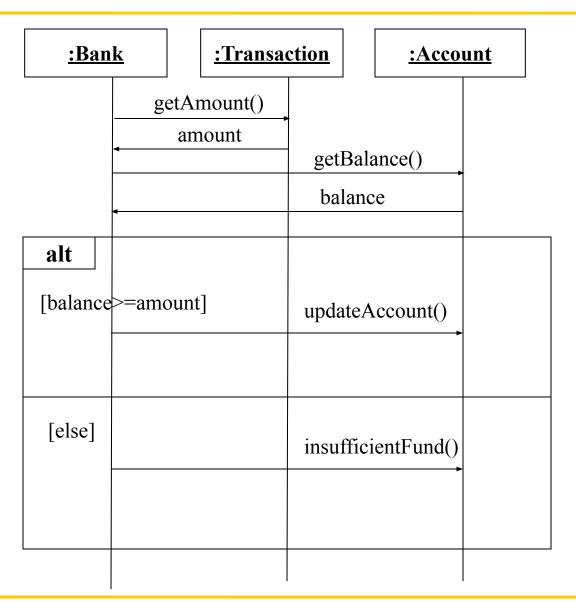
Frames can be used to specify conditional behavior (as seen in the example), loops, optional behavior etc. in sequence diagrams
